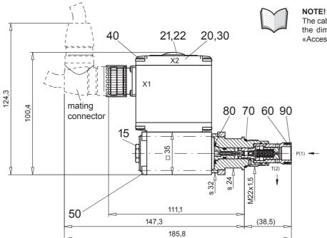
The cable connector is not part of the delivery. Regarding the dimensions see also the connector in the chapter «Accessories».
