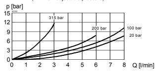
Q<sub>I</sub> = f (p) Leakage volume flow characteristics
