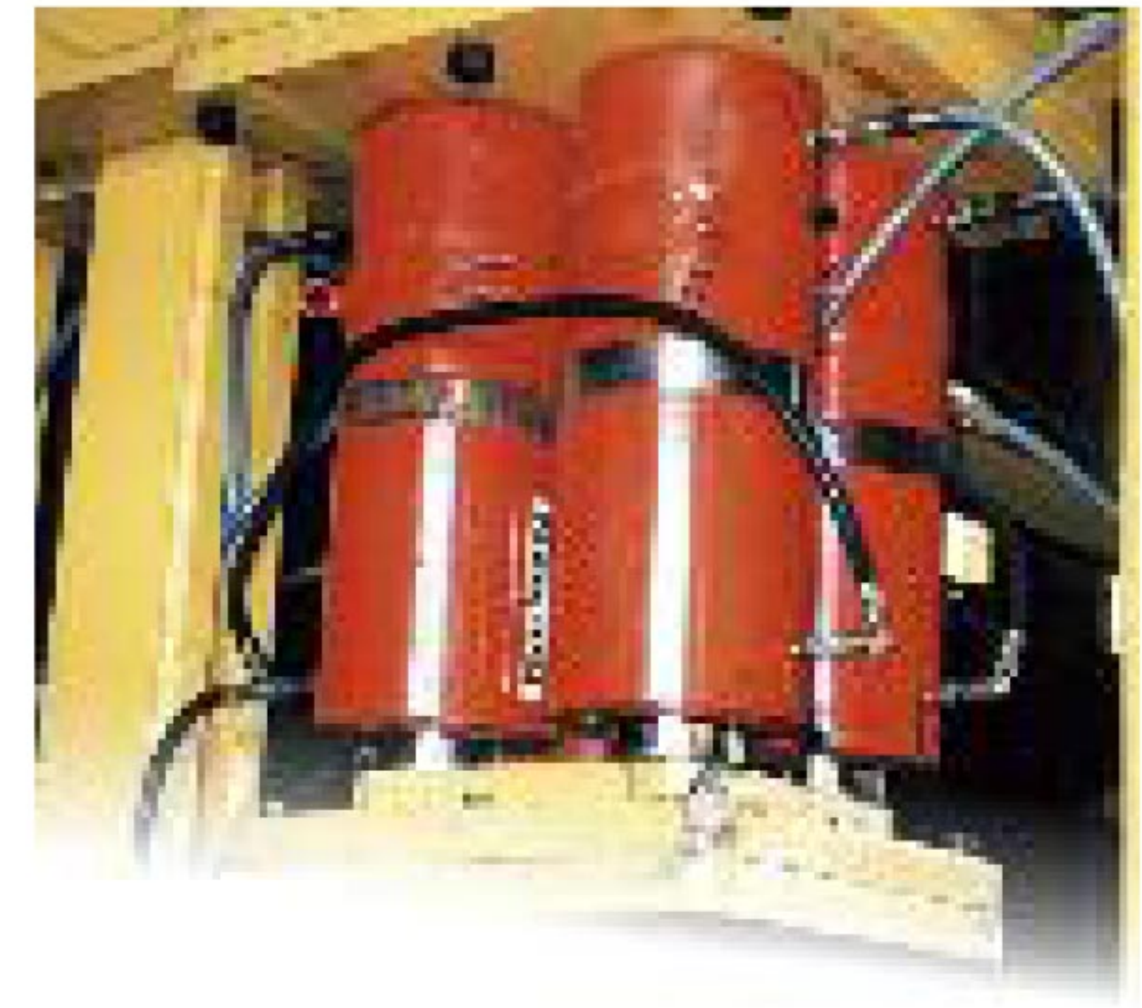
Four special order 500 ton, 24" stroke cylinders used in a swaging press for crimping 3 1/2" wire rope.
