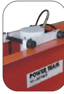
Cylinder is easily moved across width of upper bolster.
