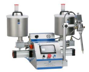
Metering Pumps: Single acting positive displacement.
