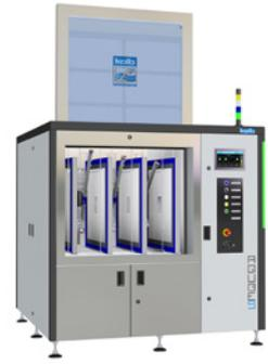
Fully automatic XXL fourfold screen / stencil cleaning system with eightfold ASYNCHRO® stainless steel rotor configuration
