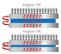
Bulk conductivity and contact resistance being equal, a thinner bond line will result
