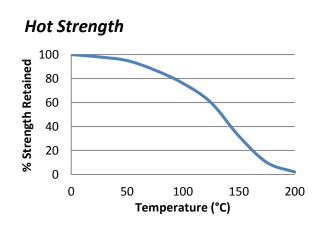
"Hot strength" shear strength tests performed on mild steel. Fully cured specimens conditioned to pull temperature for 30 minutes before testing at temperature.
