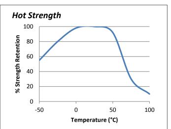
"Hot strength" shear strength tests performed on mild steel. 24hr cure at room temperature and conditioned to pull temperature for 30 minutes before testina.
