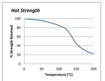
"Hot strength" shear strength tests performed on mild steel. Fully cured then conditioned to pull temperature for 30 minutes before testing. ES5741 can withstand higher temperatures for brief periods (such as for paint baking and wave soldering processes) providing the joint is not unduly stressed. The minimum temperature the cured adhesive can be exposed to is -40°C (-40°F) depending on the materials being bonded.
