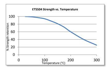
ES5504 can withstand higher temperatures of up to  $300^{\circ}$ C (570°F) providing the joint is not unduly stressed. The minimum temperature the cured adhesive can be exposed to is -40°C (-40°F) depending on the materials being bonded.
